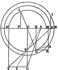
of the angle KNR or BCL to the radius KN=DI=AC, each of these lines being equal to the sine of BI; the line QM therefore varies as the velocity, and will always be equivalent to the friction, provided that it be once equivalent to it, as it is supposed to be at A; the ratio of the forces concerned, in any two succeeding instants, being always such as to maintain a regular vibration.
